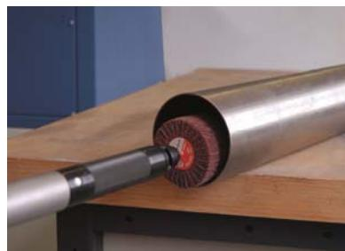
The idea is as simple as it is ingenious: extensions that are connected between the flexible shaft and the tool.
