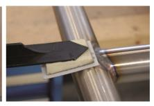
By using hook and loop attachment of abrasive pads and surface conditioning pieces, the UMC 6-R Lcan quickly solve any finishing application. Suhner's wide range of loop backed abrasives can be rapidly applied.
